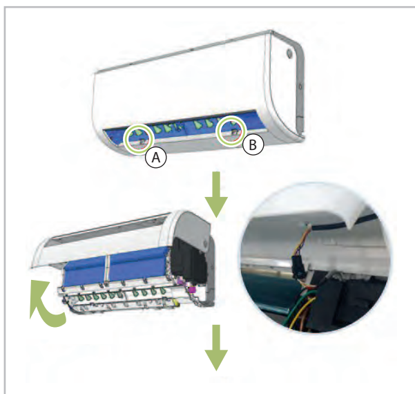
Fig. 46: Remove the screws
