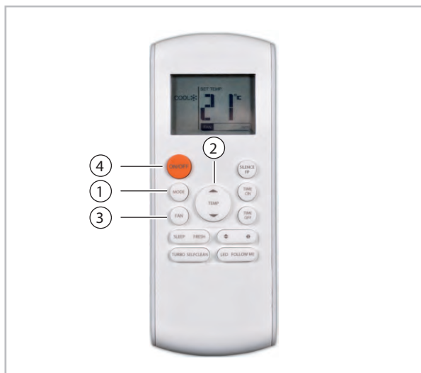
Fig. 21: "Cooling", "Heating" and "Recirculation" mode
