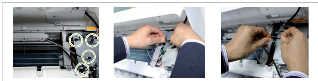
Fig. 57: Connect with the display and control board
