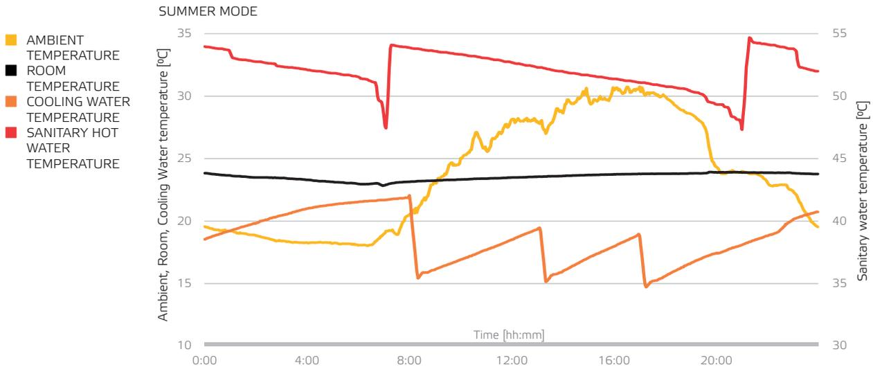
Graph representing influence of ambient temperature to the indoor temperature. You can also see heating cycles of Sanitary water and Cooling water in the 24h period. Even in a hot summer day, our heat pump had to only start 3 times, which is really helpful in order to achieve higher lifespan of the device and lower cooling expenses.
